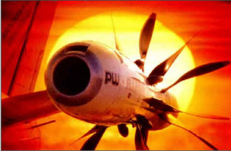
The P&W/Alison 578-DX (the Propfan™ engine with a reduction gearbox driving the propellers)
