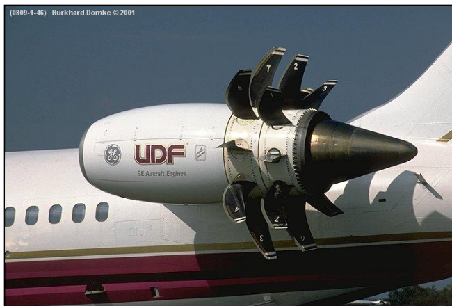
The General Electric GE-36 (the UDF™ with direct drive contra rotating propellers)
