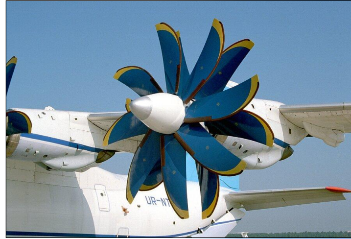
The Progress-D27 (a forward counter-rotating open rotor engine made for the Antonov-70).
